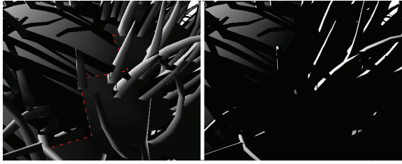
Figure 8: With standard vertex normals, light leaks in back-faces (red line). We bend normals for coherent shading.
